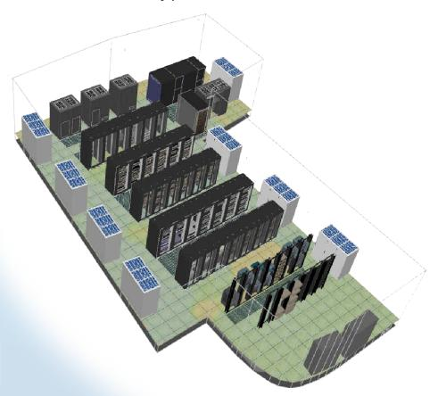
The custom-built VF provides an accurate and holistic perspective, allowing the data centre operator to track past events, investigate the present status and predict the impact of future changes, with no risk to the real facility.
